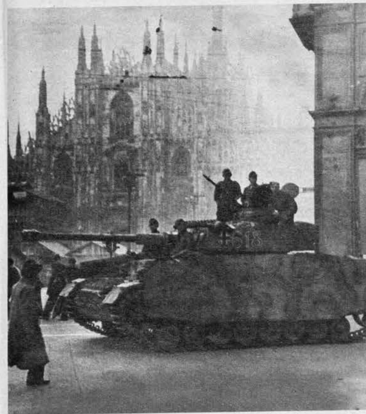
Prominent armored skirting on Mark IV conceals and protects hull and suspension system. Turret looks larger in diameter with added armor. Prominent cupola is German feature, as is muzzle brake on gun.
